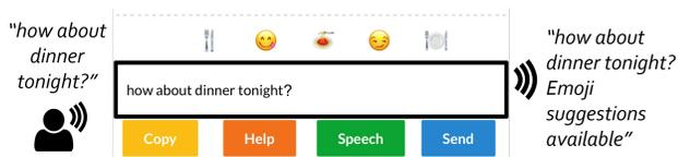
**Figure 6: When no emoji command is received, five emoji suggestions are produced by Voicemoji based on the spoken word content. For example, for the phrase, “how about dinner tonight?”, Voicemoji produces a fork and knife emoji, smiley face licking its lips emoji, plate of spaghetti emoji, smirking face emoji, and dinner plate with utensils emoji.**
