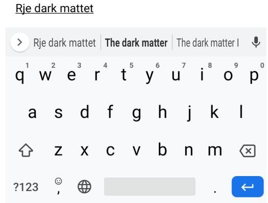
**Figure 2: The interface of PhraseFlow v1.0. The keyboard layout was the same as Gboard. The typed text here is *Rje dark mettet*, and the autocorrection candidate *The dark matter* is in bold. Three candidates are shown in the list: the literal string, the autocorrection candidate, and the second best candidate**
